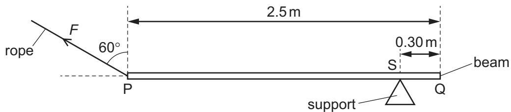
A rope is attached at one end of the beam. The rope is at an angle of  $60^\circ$  to the vertical and exerts a force  $F$ , in newtons, on the beam.
