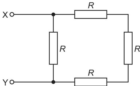
The total resistance between point X and point Y is  $120\Omega$ .
